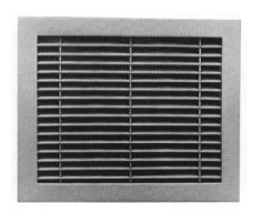
The SEC-3 is constructed with a 14 gauge steel frame and 1/8" x 1/2" blades on 1/2" centers supported by 14 gauge vertical bars on 6" centers. Blades can be fixed at 0,15, and 40 degree deflection. A 14 gauge sleeve, 11/2" long for floor grilles, is welded to face plate. Sleeves can be various depths to accommodate wall and ceiling constructions. Factory primed gray or white.
