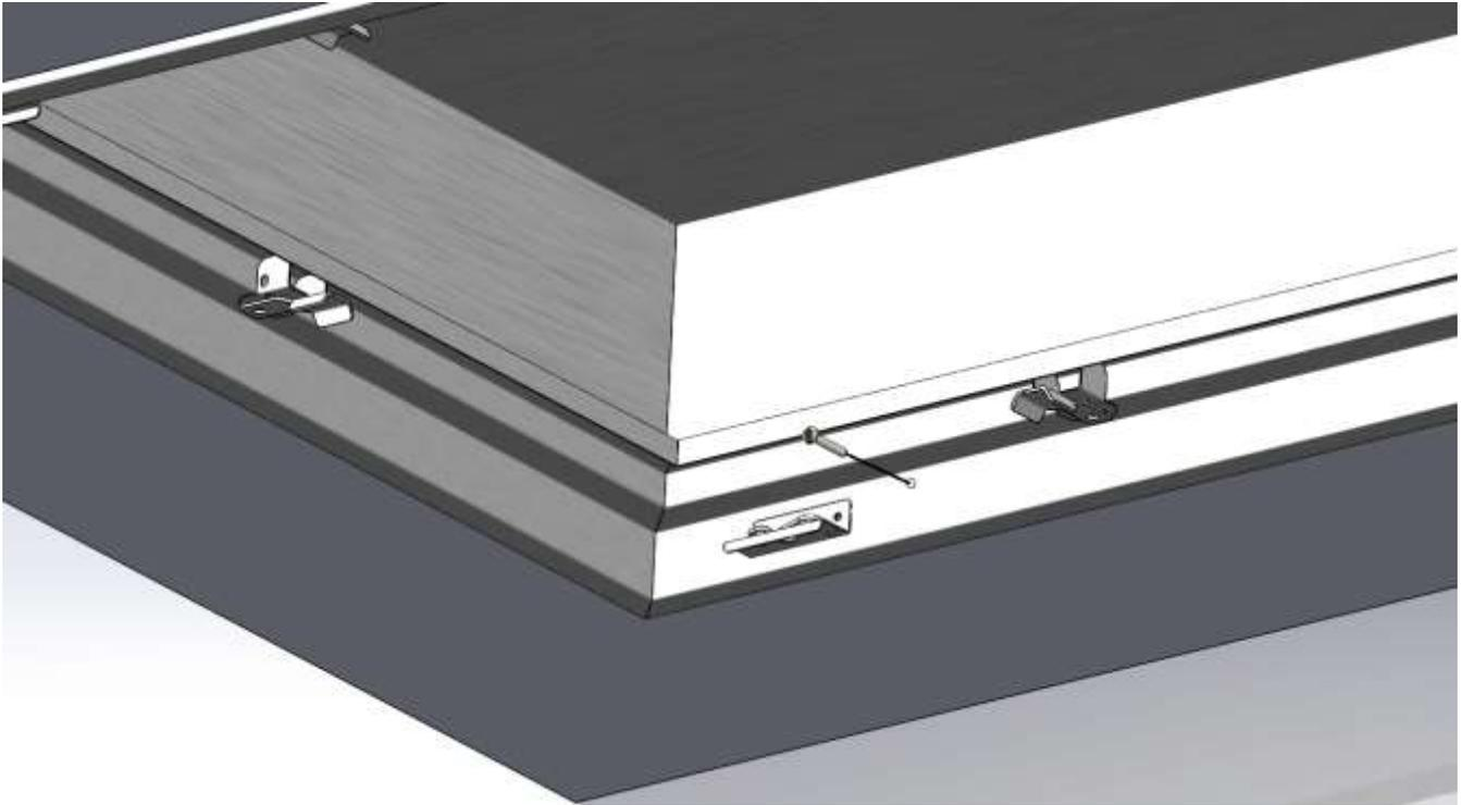
Step 7 -- Install duct work as required. Clean installation debris from the unit and surrounding ceiling.
