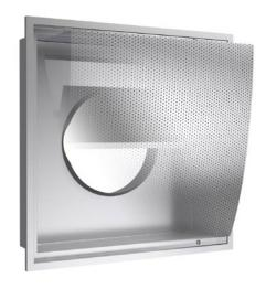
The HRDP diffuser is designed to provide low aspiration and high ventilation rates. The unique design of solid baffles in an intrusive perforated face can handle large volumes of air with low initial face velocities. The face of the diffuser is attached to the plenum with stainless steel hinges, and the opposite side is secured with 1/4-turn fasteners, allowing easy access to the interior for cleaning and sanitation.
