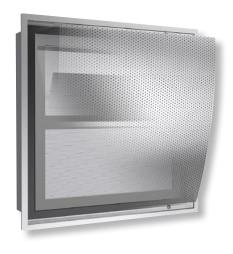
The HRDP is designed to provide low aspiration and high ventilation rates. The unique design of solid baffles in an intrusive perforated face can handle large volumes of air with low initial face velocities. The face of the diffuser is attached to the plenum with stainless steel hinges, and the opposite side is secured with 1/4-turn fasteners, allowing easy access to the interior for cleaning, sanitation and filter changes.
