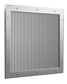
The Egg Crate Series provides 90% free area. Bars are 24-gauge type 304 stainless steel in a  $\frac{1}{2}$ " x  $\frac{1}{2}$ " x  $\frac{1}{2}$ " grid core. Type 316 stainless steel is available at additional cost. The egg crate core offers a large opening area for return air flow. Other blade sizes and spacings are also available.
