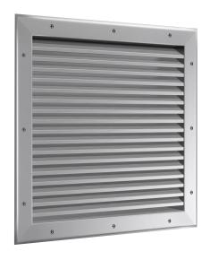
The SSDL Deep Louvered Return Grille is a non-adjustable 1-1/2" deep return grille made with louvered blades for limited vision on exterior applications. The blades are reinforced from the rear on approximate 12" centers.
