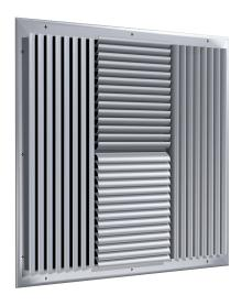
SSCB Curved Blade Supply Grille presents a clean, functional, strong appearance, along with high performance. It is designed for ceiling, high side wall, and low side wall installations. Excellent for variable air volume applications. It is available in 1, 2, 3, or 4-Way directional airflow configurations. SSCB louvers are spaced on 0.75" centers and individually adjustable from the face of the diffuser. Wide selection of duct sizes to choose from.
