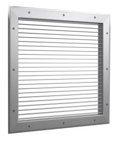
The Series 550 Return Air Grille is styled to match the 150 and 250 Supply Grilles. The face blades are non-adjustable and available in either a horizontal position (550H) or vertical position (550V), factory set at either 0° or 45° degrees, spaced on .75" centers. The same hollow air-foil blades used on the supply grilles are used on the return air grilles.
