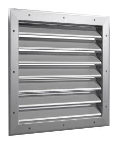
The 550 LT Series Long Throw Return Air Grille is styled to match the 150 and 250 Supply Grilles. The face blades are non-adjustable and available in either a horizontal position (550H LT) or vertical position (550V LT), factory set at either 0° or 45° degrees, spaced on 1.5" or 3" centers, with custom configurations available at an additional cost. The same hollow air-foil blades used on the supply grilles are used on the return air grilles.
