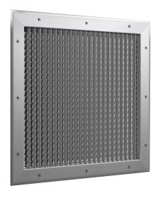
The 250 Series Double Deflection Supply Grille provides effective directional control of the air stream in one, two, three or four directions. Each bank of blades is pivoted at the front which gives a uniform appearance regardless of blade angle setting. The hollow air-foil grille blades are spaced on .75" centers. Each blade is adjusted for the desired air deflection without affecting the setting of any other blade. Available with horizontal face blades (250-H) or vertical face blades (250-V).
