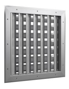
The 250 LT Series Long Throw Double Deflection Supply Grille provides effective directional control of large volumes of air flow. Each blade is pivoted which allows for custom air flow. The deflector blades are spaced on 1½" or 3" centers. Each blade is adjusted for the desired air deflection without affecting the setting of any other blade. Available with horizontal face blades (250H LT) or vertical face blades (250V LT).
