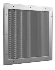
The 250 HD Series Heavy Duty Double Deflection Supply Grille provides effective directional control of the air stream. The hollow, air-foil grille front blades are set at a fixed at 0° or 45° on .5" centers. Back blades are spaced on .75" centers and each blade is individually adjusted for the desired air deflection without affecting the setting of any other blade. Available with horizontal face blades (250HD-H) or vertical face bars (250HD-V).
