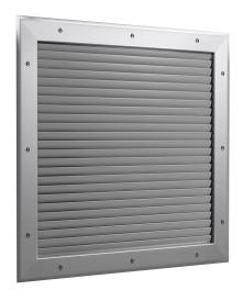
The 150 Series Single Deflection Supply Grille provides effective directional control of the air stream in one or two directions. The blades are pivoted at the face, giving a uniform, aligned appearance regardless of blade angle setting. The hollow, air-foil grille blades are spaced on .75" centers. Each blade is adjusted for the desired air deflection without affecting the setting of any other blade. Available with horizontal face blades (150-H) or vertical face blades (150-V).
