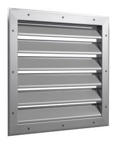
The 150 LT Long Throw Supply Grille provides effective directional control of large volumes of air flow. Each blade is pivoted, which allows for custom air flow. The deflector blades are spaced on either 1.5" or 3" centers, as specified. Each blade is adjusted for the desired air deflection without affecting the setting of any other blade. Available with horizontal face blades (150H LT) or vertical face blades (150V LT).
