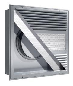
These diffusers feature an adjustable pattern control technology – using adjustable blades which hang less that 1 below the ceiling – to deliver high volumes of low velocity air in a radial pattern. Two versions are available: with a perforated center section or with an optional adjustable face. Both versions can be configured with an extended plenum and unique frame design to accommodate a gel seal HEPA or ULPA filter. Filters can be easily removed and replaced from the face of the unit.
