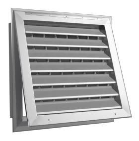
The SSHFG 250 LT Series Long Throw Double Deflection Hinged Filter Grille is hinged in our 1000 Plaster Frame and secured with low profile ½-turn fasteners. The hinged filter grille allows easy access to filters or mechanical equipment. It provides effective directional control of large volumes of air flow. Each blade is pivoted which allows for custom air flow.
