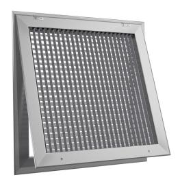
The SSHFG 250 Series Double Deflection Hinged Filter Grille is hinged in our 1000 Plaster Frame and secured with low profile ¼-turn fasteners. The hinged filter grille allows easy access to filters or mechanical equipment. It provides effective directional control of the air stream in one, two, three or four directions. Each bank of blades is pivoted at the front which gives a uniform appearance regardless of blade angle setting.
