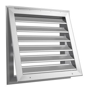
The SSHFG 150 LT Long Throw Single Deflection Hinged Filter Grille is hinged in our 1000 Plaster Frame and secured with low profile 1/4-turn fasteners. The hinged filter grille allows easy access to filters or mechanical equipment. It provides effective directional control of large volumes of air flow. Each blade is pivoted, which allows for custom air flow.
