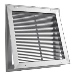
The SSHFG 550 HD Heavy Duty Single Deflection Hinged Filter Grille is hinged in our 1000 Plaster Frame and secured with low profile ¼-turn fasteners. The hinged filter grille allows easy access to filters or mechanical equipment. Face blades are non-adjustable and available in either a horizontal position (H) or vertical position (V), factory set at either 0° or 45°, and spaced on .750" centers.
