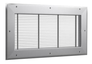
The SSLBG Series Linear Light Duty Bar Grille is designed for supply or return air in sidewall or sill installations. Designed with fixed 0° air foil blades parallel to the grille's long dimension, blades are reinforced on approximate "centers. Air foil blades are set at 0° on 3/8" centers allowing 1/4" spacing between blades.
