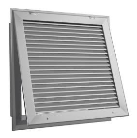
The SSHFG SSG Louvered Hinged Filter Grille is hinged in our 1000 Plaster Frame and secured with low profile ½-turn fasteners. The hinged filter grille allows easy access to filters or mechanical equipment. It is a non-adjustable return grille made with louvered blades for limited vision or exterior applications, and set within our Hinged Filter Grille. The blades are reinforced from the rear on approximate 12" centers.
