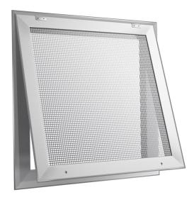
The SSHFG PERF Perforated Hinged Filter Grille is hinged in our 1000 Plaster Frame and secured with low profile ¼-turn fasteners. The hinged filter grille allows easy access to filters or mechanical equipment. It has a standard 51% free area on the face and can be used as a matching return in conjunction with perforated supply diffusers.
