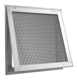
The SSHFG EC Series  $\frac{1}{2}$ " x  $\frac{1}{2}$ " Egg Crate Hinged Filter Grille is hinged in our 1000 Plaster Frame and secured with low profile  $\frac{1}{4}$ -turn fasteners. The hinged filter grille allows easy access to filters or mechanical equipment. It is constructed from type 304 Stainless steel, with #4 satin finish standard.
