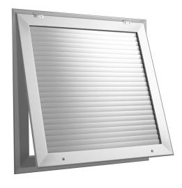
The SSHFG 150 Series Single Deflection Hinged Filter Grille is hinged in our 1000 Plaster Frame and secured with low profile ¼-turn fasteners. The hinged filter grille allows easy access to filters or mechanical equipment. It provides effective directional control of the air stream in one or two directions. The blades are pivoted at the face, giving a uniform, aligned appearance regardless of blade angle setting.
