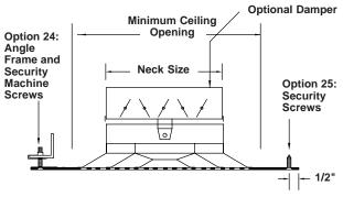
Diffuser tack welded to rear of face plate
